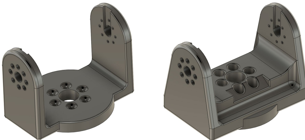
Figure 5. Improvement of the HIP_YAW link. Left: Original, Right: Redesigned structure
