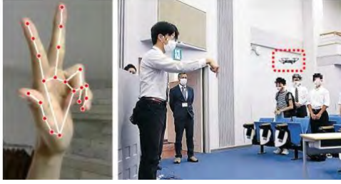
Fig. 9 showcases a drone interfacing system controlled by hand signs using a machine learning-based skeleton extraction model. The left image illustrates skeleton extraction from drone-transmitted video for hand sign detection. The right image depicts a lecture on SDGs and drone technology delivered to high school students on June 18, 2023 environmental impact. The latest challenge in air transport, particularly highlighted by drone technology, offers hope for improving sustainability. However, numerous challenges remain to overcome, such as increasing per-unit transport capacity, adapting to changes in the natural environment, ensuring safety, enhancing battery capacity, and developing infrastructure for charging stations.
