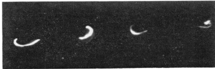
d=20\text{mm} , u=1.08\text{cm/sec} Re=348
