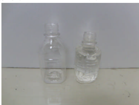
Fig.1 Appearance of thermal deformation after boiling water is injected into the non-heat resistance PET bottle (proposition from YORKEY CO. LTD)
