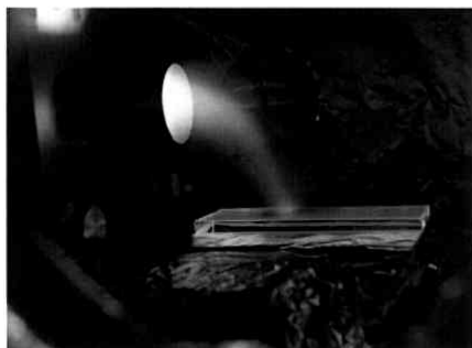
Fig.11 Deposition of Ni by magnetically deflected plasma.
