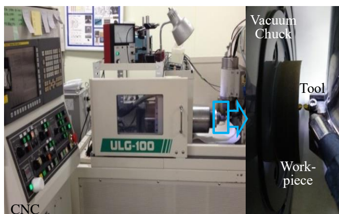
Fig. 5.4 Linear motor driven 4-axis (X, Y, Z, C) controlled ultraprecision turning machine
