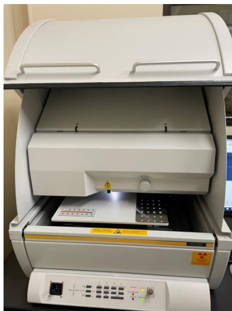
Fig 2.14 Fluorescence X-rays film thickness measurement equipment
