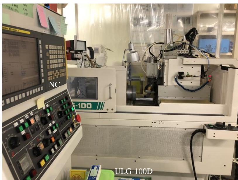
Fig. 4.2 View of linear motor driven 4-axis (X,Y,Z,C) controlled ultraprecision machine
