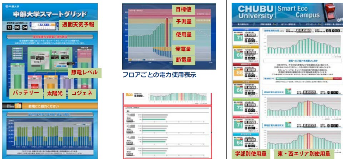
Figure 1.7 Smart grid monitor displaying the status of energy consumption in Chubu University in the real time. Figure adopted from [7].
