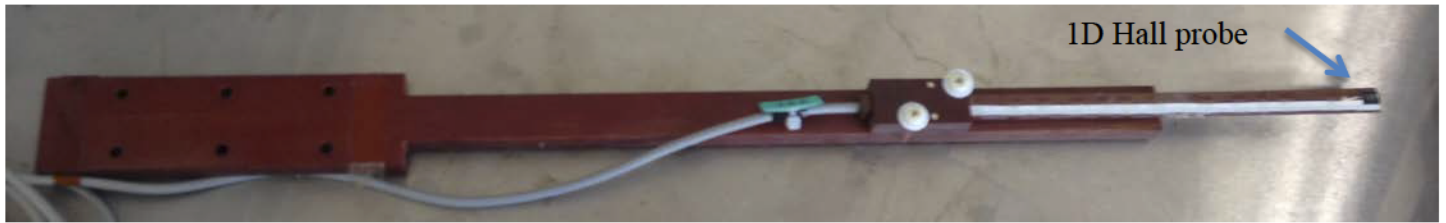
Fig. 32 Plate of the 1D Hall probe sensor.
