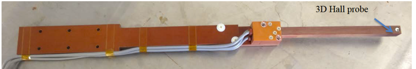
Fig. 33 Plate of the 3D Hall probe sensor.
