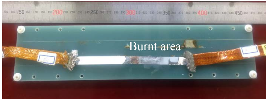
Fig. 40 Burnt Fujikura tape after over-current pulse application.
