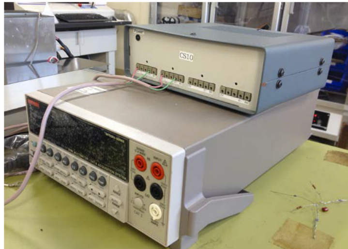
Fig. 34 Hall probe current source (up) and Keithly instrument (down).
