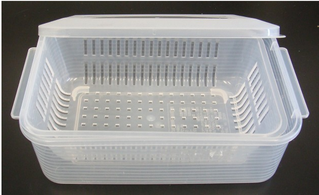
Figure 2.3 : Plastic containers used for soil burial biodegradation tests.
