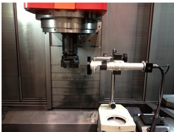
Fig.4.29 The method of tool wear observation in multi-functional machine tool
