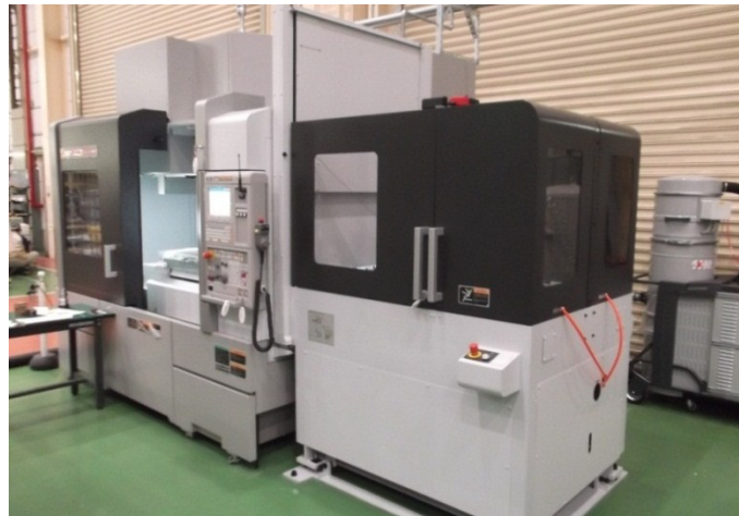
Fig.6.8 The overview of vertical machining center NVX5080 II with chip vacuum system
